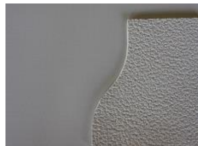
Dachmaterial thermograu, ca. 4 mm dick, 1.550 g/m 2
