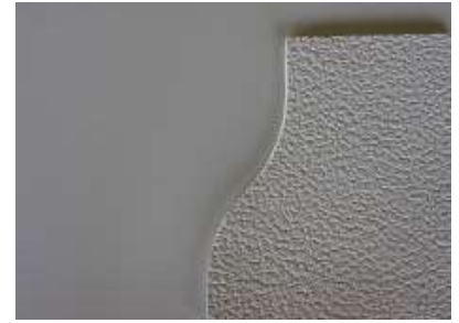
Dachmaterial thermograu, ca. 4 mm dick, 1.550 g/m 2
